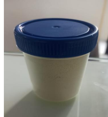
Fig. 2 Synthesised PAC from used beverage cans
